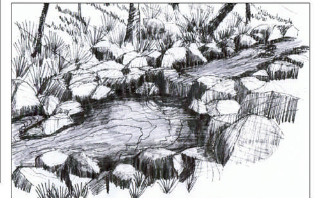
D | Drop structure using indigenous rock construction.
