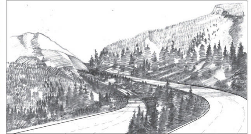
A | The existing landscape should appear to extend across the transportation corridor. Clusters of trees and other plant material representative of the life zone should be planted in the median space to accomplish this.
